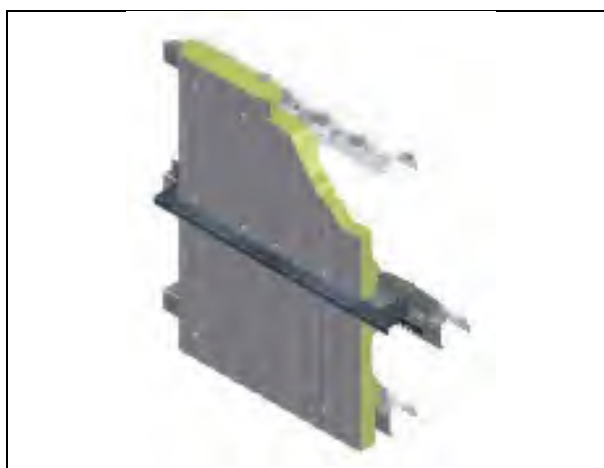
Abbildung 2-28: Stahl-Sandwichelement (Wand) Figure 2-28: Steel sandwich panel (wall)
