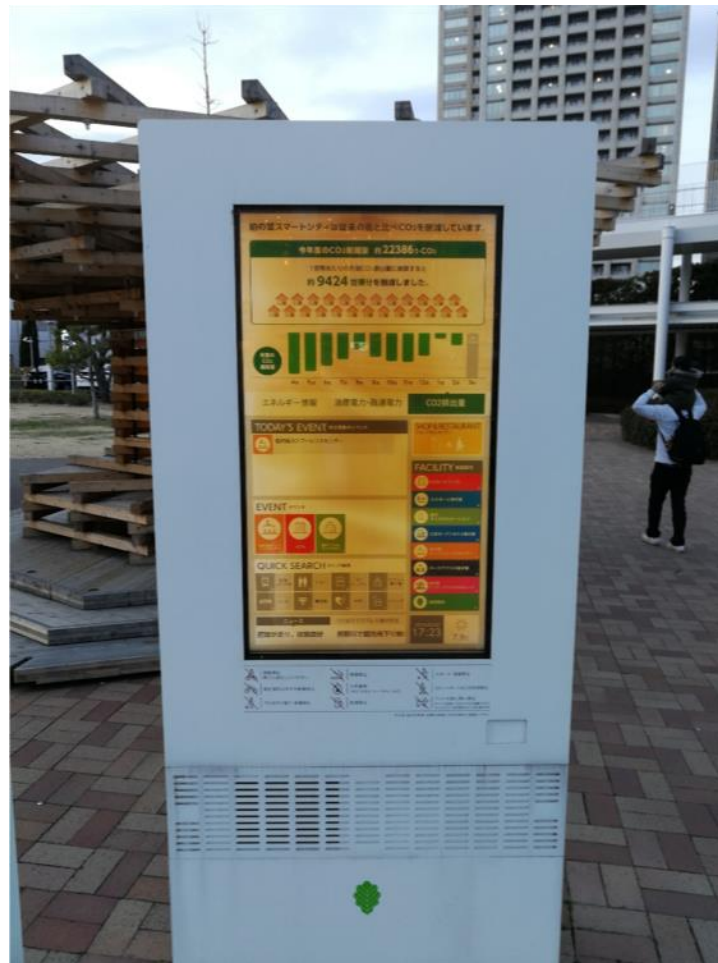
Figure 21 Public digital signage at Gate Square, Kashiwa-no-ha, showing energy consumption and carbon-dioxide emission data (Own picture).
