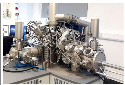
Time-of-Flight Secondary Ion Mass Spectrometry (ToF-SIMS) equipment
