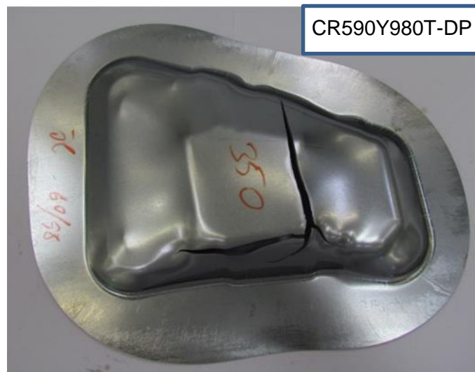
Abbildung 6-6: CR590Y980T-DP, BSU-Bauteil, Niederhalter Kraft: 350 kN, Ziehtiefe: 44 mm, Öl Figure 6-6: CR590Y980T-DP, BSU-Part, blankholder force 350kN, Drawing depth: 44 mm, lubrication oil
