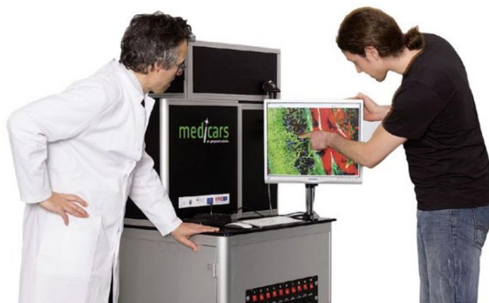
3) In the MediCARS project, funded by the German Ministry of Research, Professor Popp's working group developed a portable microscope. This can be used to measure multi-modal images in a clinical environment (coherent anti-stokes Raman scattering, second harmonic generation and two-photon excited auto-fluorescence). Using image analysis algorithms, quantitative clinical information can be extracted from these measurement data (Copyright: Leibniz-IPHT / Sven Döring)
