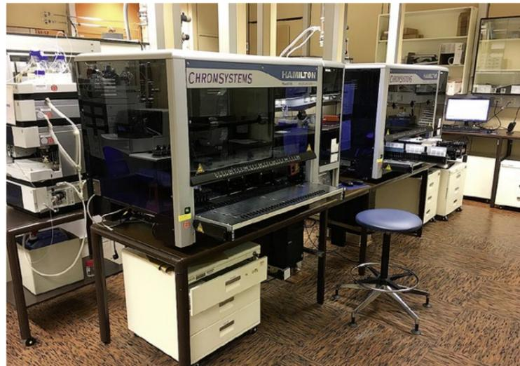
A fully automated robotic system for the determination of immunosuppressants in Stimpfl's laboratory
