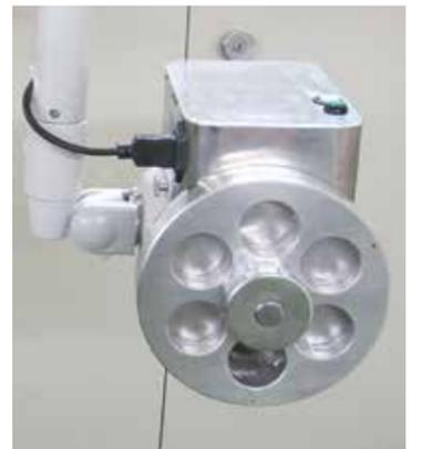
The ScreenAir device measures and quantifies the potential for aero-biocontamination during surgery
