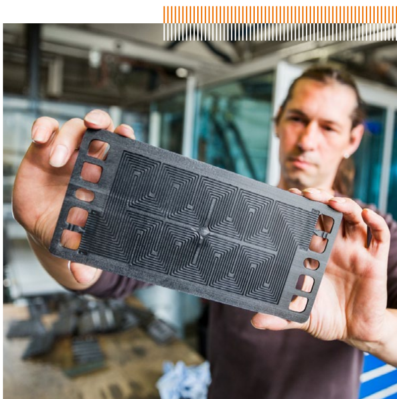
Injection-moulded bipolar plate for HT-PEFC
