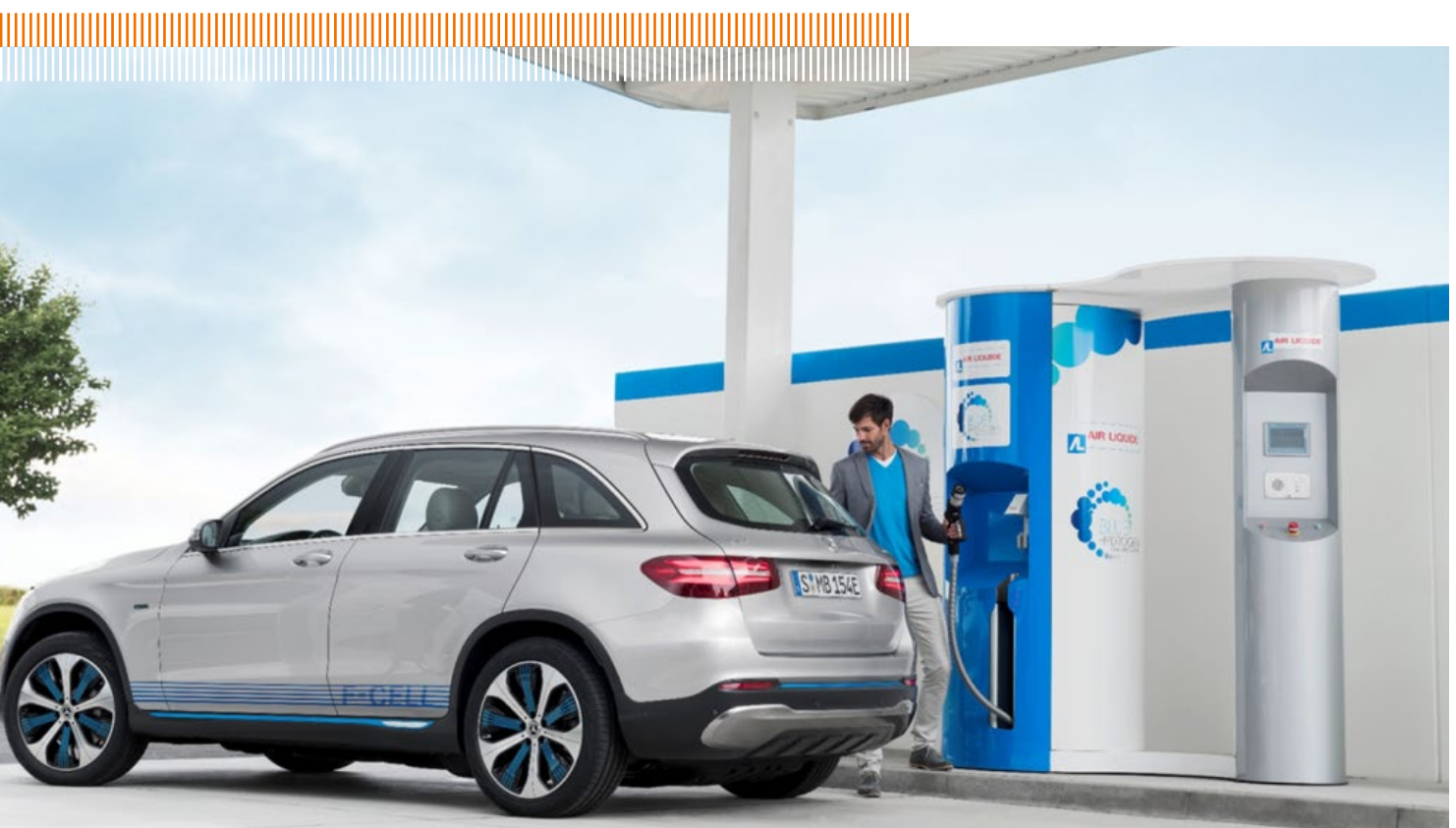
Mercedes Benz GLC F-Cell (pre-series, 147 kW electric drive, Li-ion battery with 13.8 kWh energy content, pressurised hydrogen storage tank (700 bar) with 4.4 kg of hydrogen)
