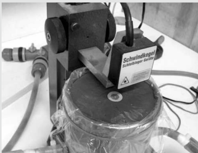
Untersuchung des autogenen Schwindens mittels Schwindkegelmethode Testing of autogenous shrinkage by shrink cone method
