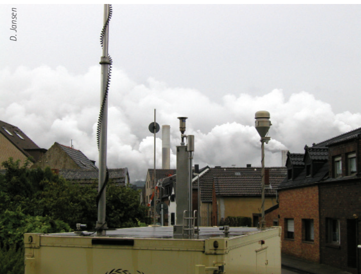
Several monitoring stations like this one in Grenbroich-Gustorf have been installed for the measurement of particulate matter.
