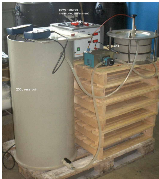
Design of the apparatus for the electrochemical destruction of cyanides. Dipl.-Ing. Angela Rheindorf
