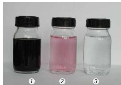
1: Coloured wastewater, 2: Filtrate of ultra-filtration, 3: Permeate of reverse osmosis
