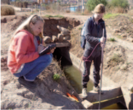
Measuring discharge in irrigation canal
