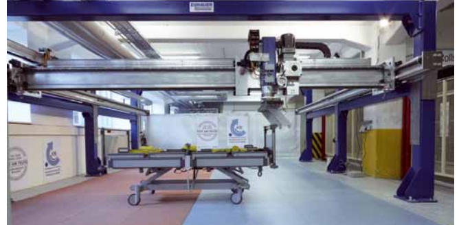
Hospital bed in the roll simulator in the test laboratory for motion analysis.
