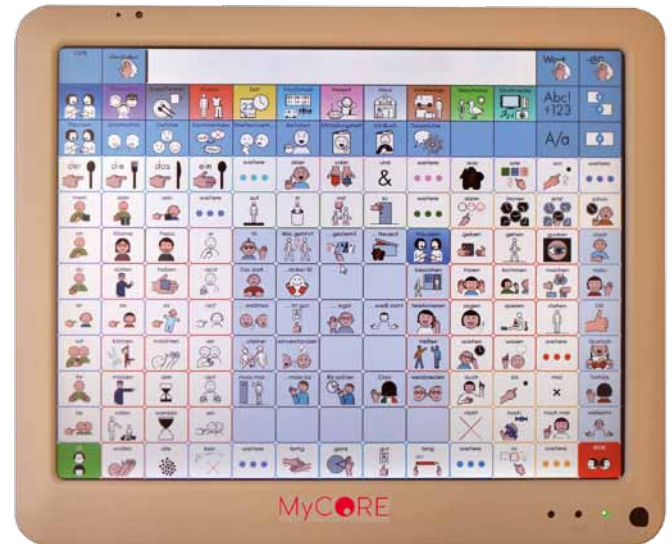
The MyCore communication aid: Symbol-based vocabulary is provided on a static frame with core vocabulary and topic/fringe vocabulary organised in categories.
