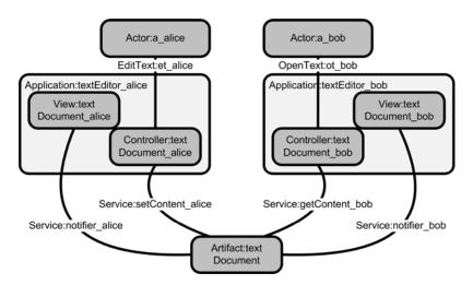
Figure 9 Decomposition of collaborative applications using the model-view-controller pattern
