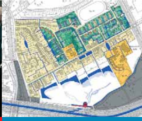
The open discharge of rain water links the just upgraded settlement with the surrounding water courses – and gives attractiveness to the houses' environment.
